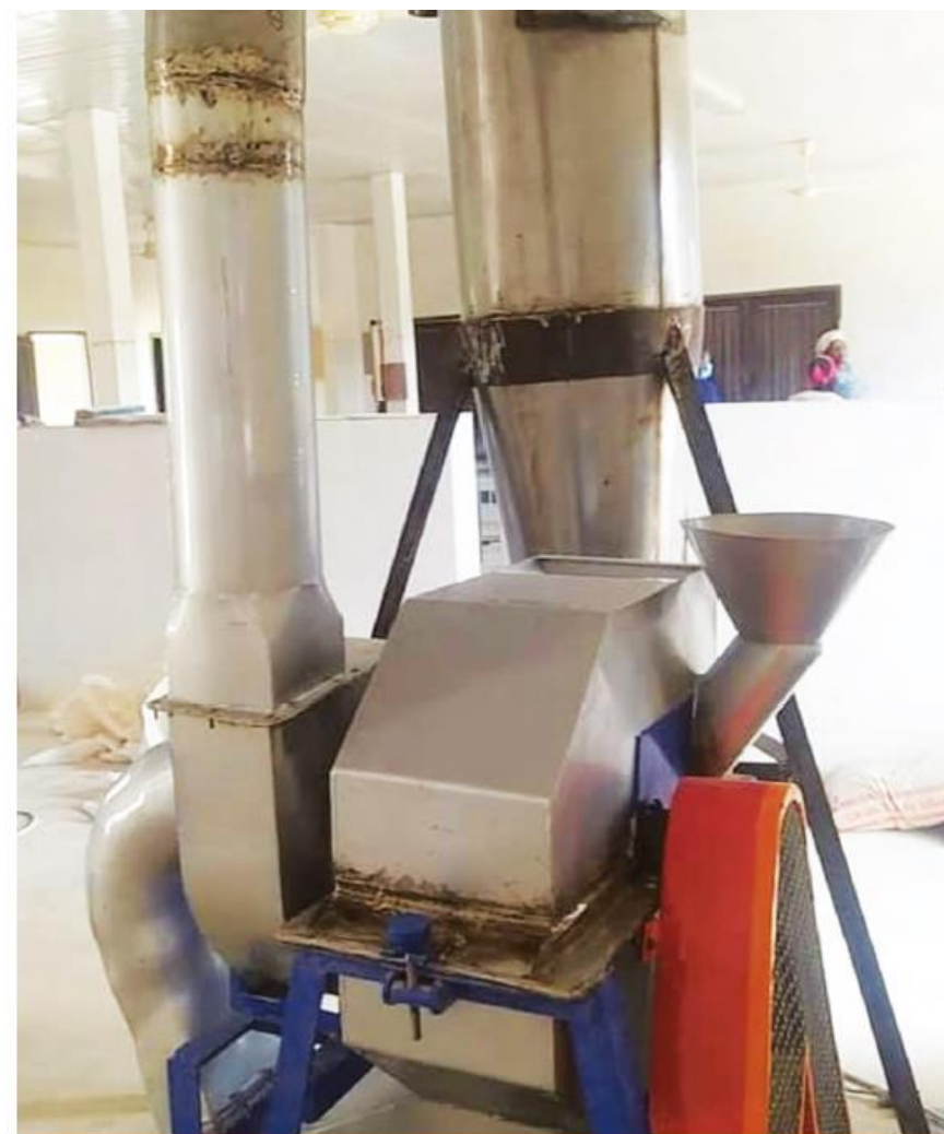
The solar-powered multipurpose hammermill at the manufacturer's premises, First Product Enterprise Ltd., in Ghana.
