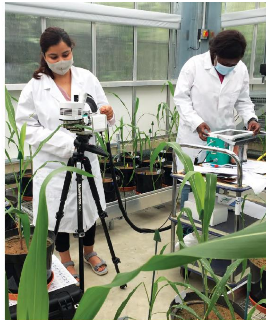
Measuring leaf-level photosynthesis and fluorescence in a greenhouse pot experiment where plant nutrition effects on Striga -infected sorghum plants are assessed, from L–R, Students: Yamuna Nuepane Ghimire (MSc) and Immaculate Mwangangi (PhD).
